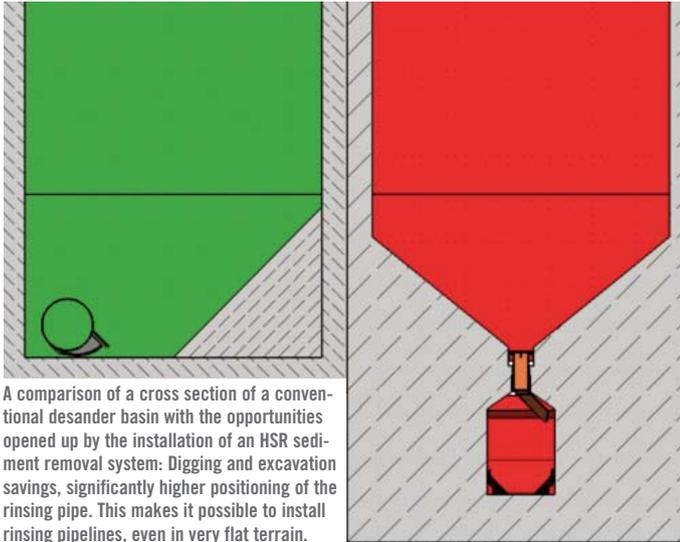
A comparison of a cross section of a conventional desander basin with the opportunities opened up by the installation of an HSR sediment removal system: Digging and excavation savings, significantly higher positioning of the rinsing pipe. This makes it possible to install rinsing pipelines, even in very flat terrain.
